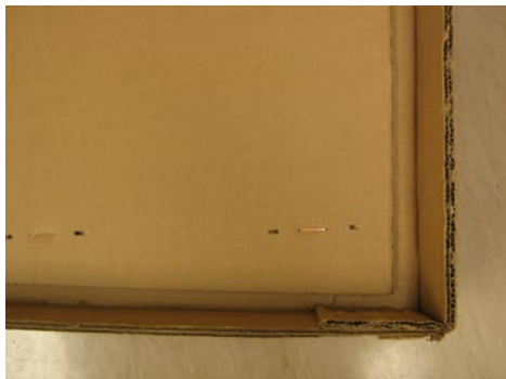
Channel around perimeter for sidewalls
