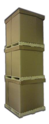
"Actual totes tested for 90 days filled with high density resin three high."
